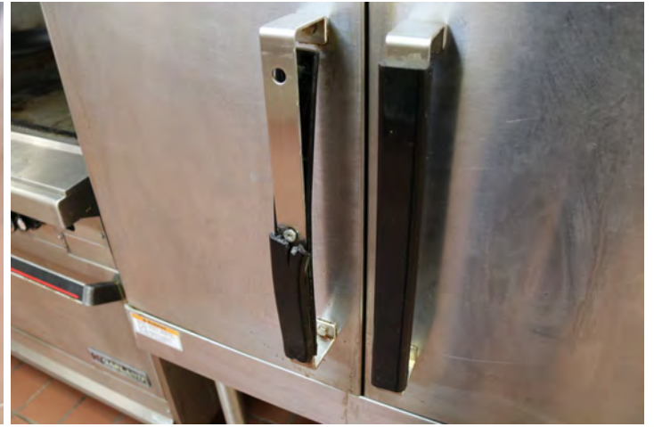
Clean exterior and replace broken handle
